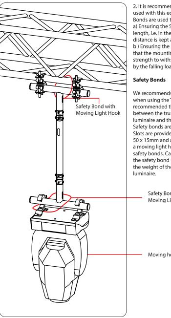
2. It is recommended that Safety Bonds are used with this equipment. When Safety Bonds are used the user is responsible for: a) Ensuring the Safety Bond is of optimum length, i.e. in the event of failure, the 'drop' distance is kept as short as possible. b) Ensuring the Safety Bond is attached so that the mounting points are of sufficient strength to withstand the forces imposed by the falling load.
